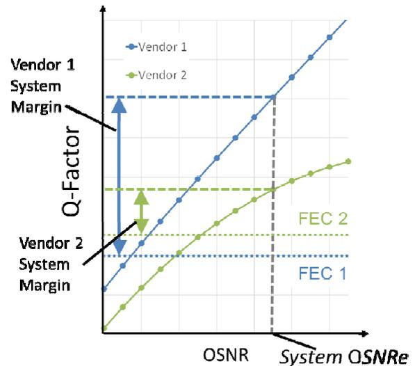
Figure 2: A reference Line card (Vendor 1) can be used to predict the performance of another line card (Vendor 2) on the same wet plant, and characterize the wet plant by evaluating its degradation.
