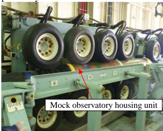
Photo 7: Trial for laying/recovery of the mock observatory unit by LCE
