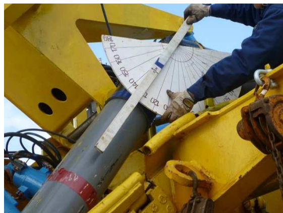
Photo 4: Measurement of the gimbal angle
