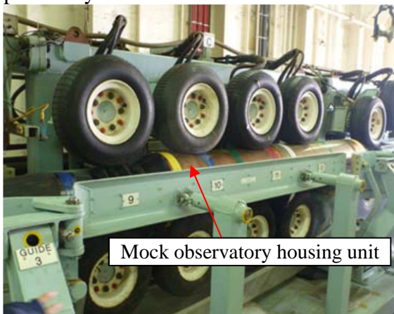
Photo 7: Trial for laying/recovery of the mock observatory unit by LCE
