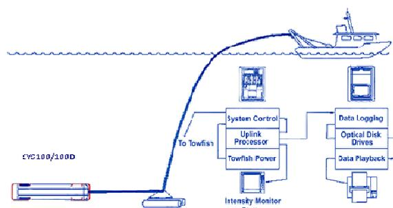
**Figure 2: Shallow water swath bathymetry system vessel and tow configuration.**
