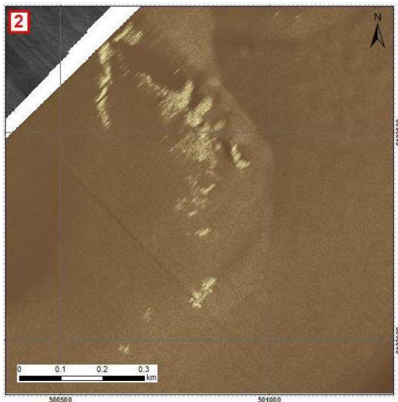
Figure 6: AUV-mounted side scan sonar data over geologic features © Fugro
