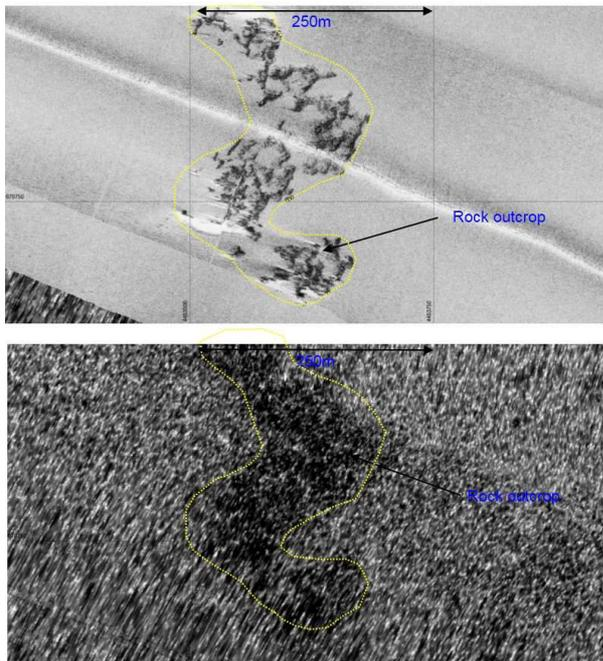
**Figure 5: Geological feature comparison between side scan sonar (top) and backscatter (bottom) data at the same scale.**
