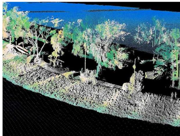
**Figure 10: Integrated bathymetry and laser scanning data at the marine/terrestrial boundary**
