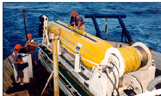
Figure 1: Deep-water swath bathymetry system being prepared for launching © Don Hussong
