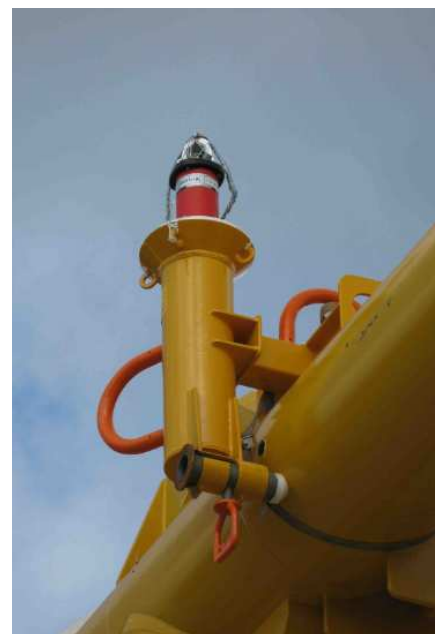
Image 4. Typical Transponder on a Subsea Structure
