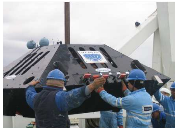
Image 5. Subsea Node used in VENUS system
