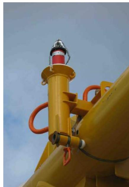
**Image 4. Typical Transponder on a Subsea Structure**
