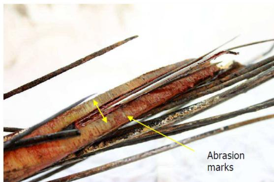
**Figure 1: Example of Abraded Cable**
