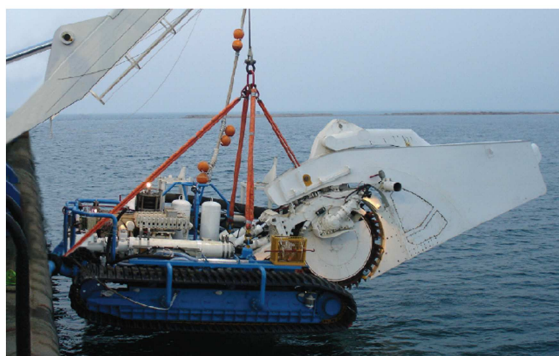
Figure 6: Typical Rock Trencher
