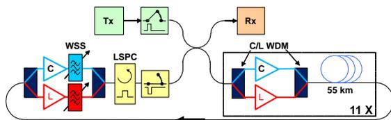
**Fig. 2. Circulating loop test bed using C+L EDFAs. LSPC: loop synchronized polarization controller, WSS: wavelength selective switch.**
