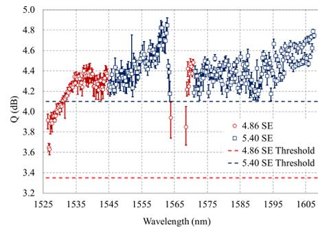
**Fig. 3: 49.3 Tb/s with 282 channels after ~9,100 km.**
