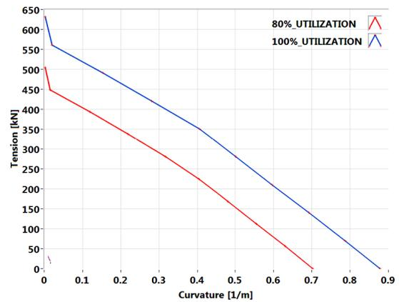
**Figure 13** Tension vs. Curvature plots in the sag region at the Gulf of Guinea location.
