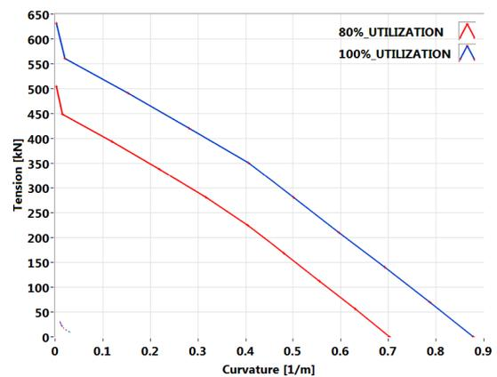
**Figure 14** Tension vs. Curvature plots in the hog region at the Gulf of Guinea location.
