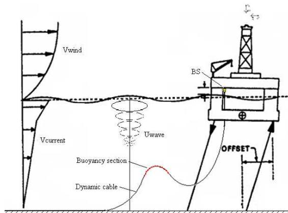
Figure 5 Vessel offset description.
