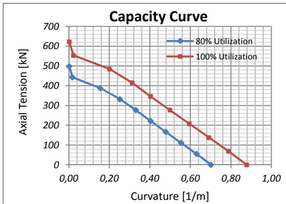
Figure 2 Capacity curve of the Dynamic FO Riser.
