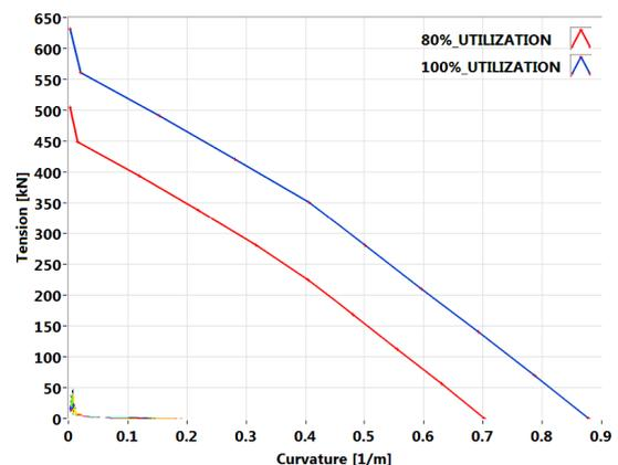
Figure 11 Tension vs. Curvature plots in the TDP region at the North Sea location.
