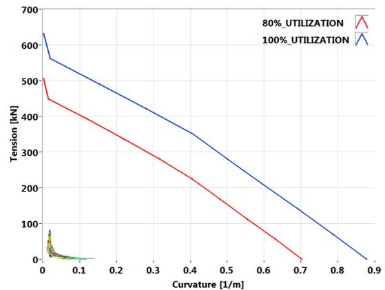
Figure 10 Tension vs. Curvature plots in the hog region at the North Sea location.
