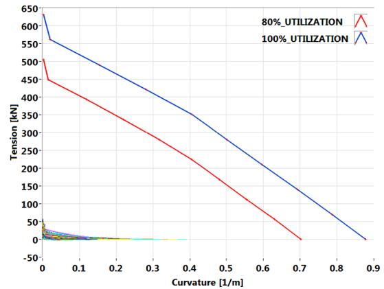
Figure 9 Tension vs. Curvature plots in the sag region at the North Sea location.
