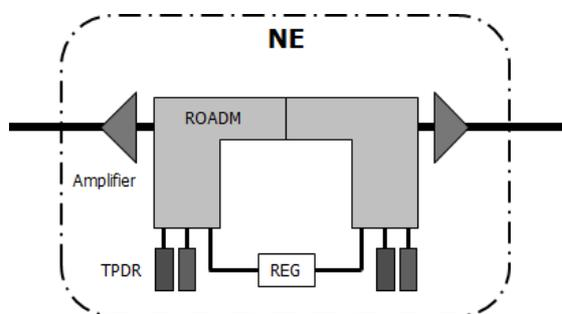
Figure 6: Cascade of 2 repeaterless spans connected via a ROADM
