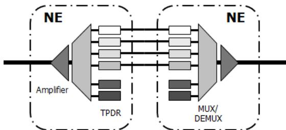
Figure 1: Back-to-back SLTEs interconnecting 2 repeaterless spans
