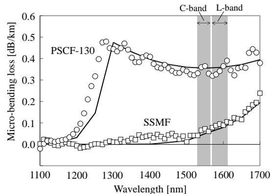
Figure 5: Micro-bending loss of PSCF-130
