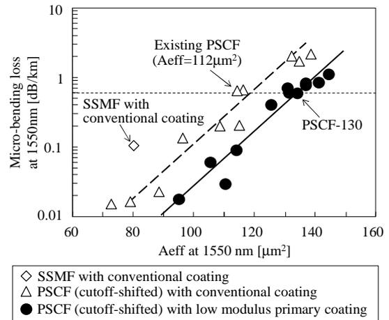
Figure 4: Effect of low modulus primary coating on micro-bending loss.
