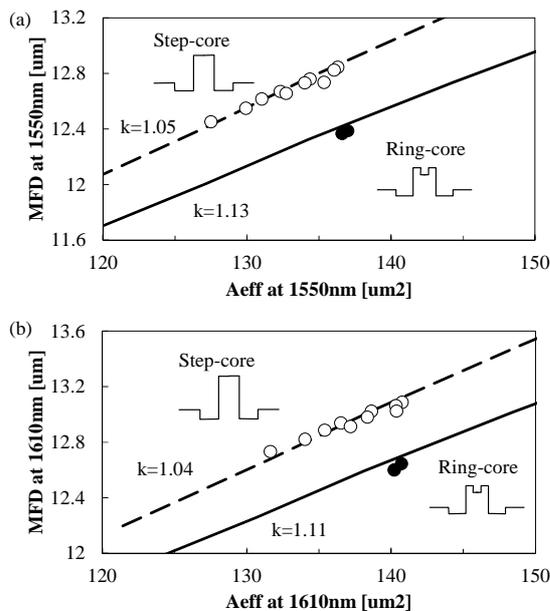
Figure 6: Reduction in MFD by ring core for low splice loss to SSMF in (a) C-band and (b) L-band.
