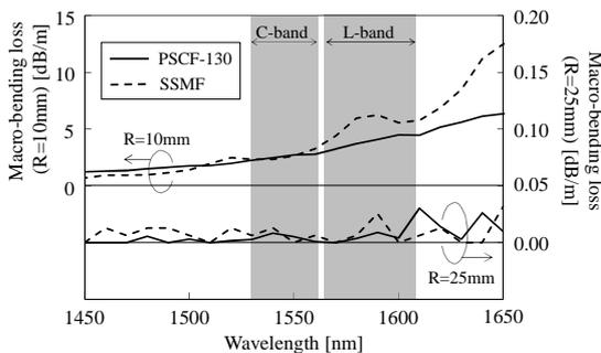
Figure 3: Macro-bending loss of PSCF-130
