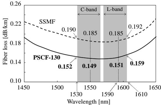
Figure 2: Loss spectrum of PSCF-130
