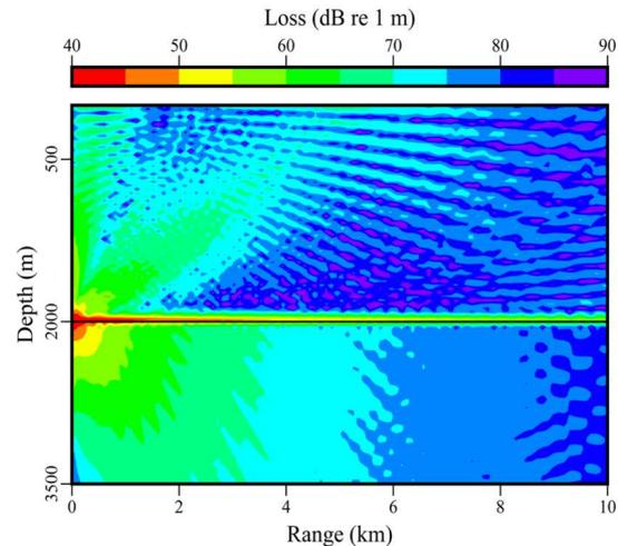
Figure 2: Interference Patterns from Acoustic Reflections [11]
