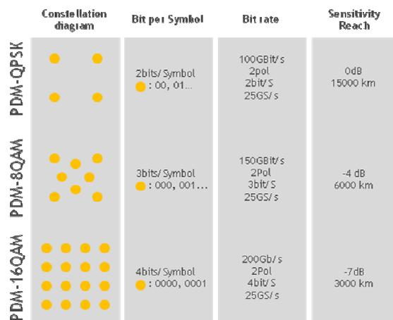
**Figure 1: Modulation formats and bit rates for a 25G Symbol/s rate**
