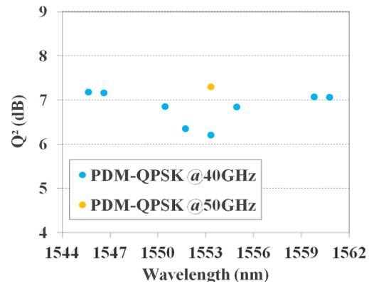
**Figure 4: Globenet segment 4 average Q<sup>2</sup> performance with 100Gbit/s PDM-QPSK**
