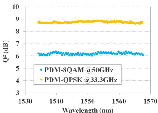
**Figure 2: PDM-8QAM @50GHz and PDM-QPSK @33.3GHz after 4000km**
