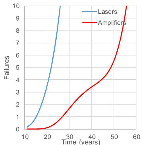
Figure 4: Failures for 500 amplifier-pairs
