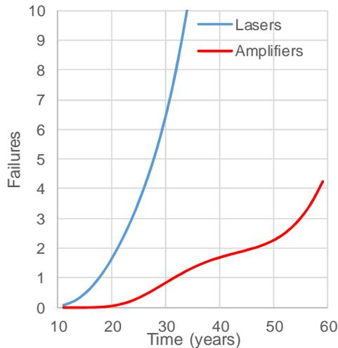
**Figure 5: Failures for 100 amplifier-pairs
