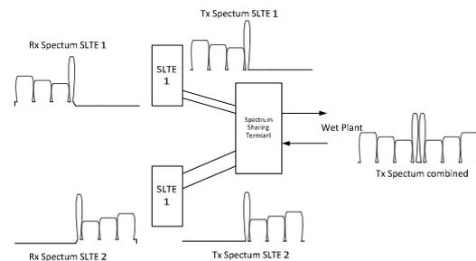
**Figure 4 Coupling via a Spectrum Sharing Terminal**
