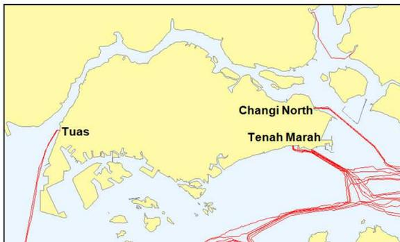
**Figure 3 Telecommunication cable landings in Singapore**
