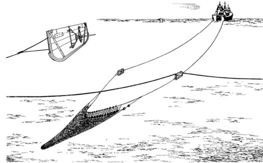
**Figure 2 Bottom Trawl Catch Cable**
