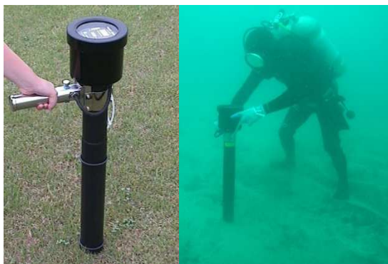
Fig. 1: Cable Probe (left), Diver with Cable Probe (right)
