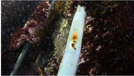
Fig. 10 : Localized Fault Point (Shunt Fault)
