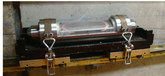
Figure 5: New ASN joint design, long length tensile test
