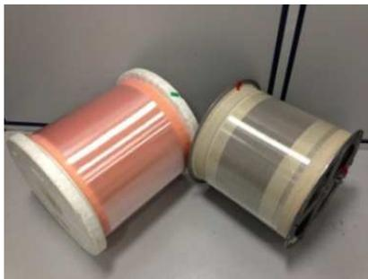
Figure 1: Microbending test spools
