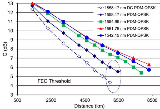
**Figure 2. Q-factor vs. Distance at optimal OSNR**
