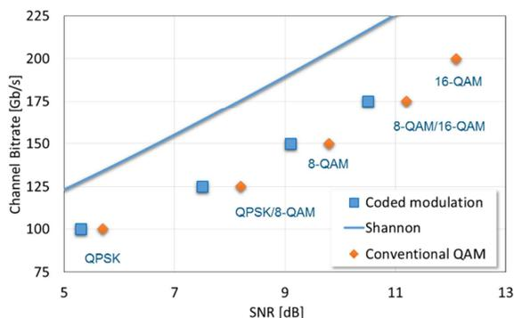
**Figure 4. Performance of Coded Modulation, Time Hybrid Modulation, and Conventional QAM.**
