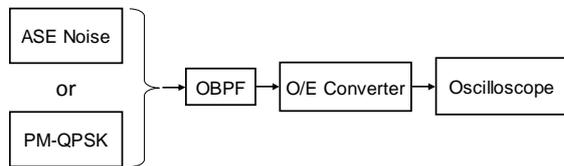
Figure 5: Setup for measuring optical power variation
